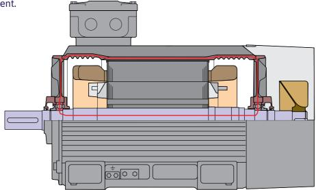
The **Shaft Current** discharges trough the bearings and motor frame.
