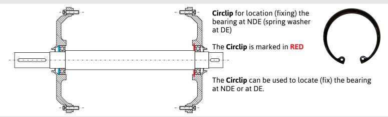
Bearings located with a Bearing Retainer plate (shaft axial movement reduced to dilatation)
