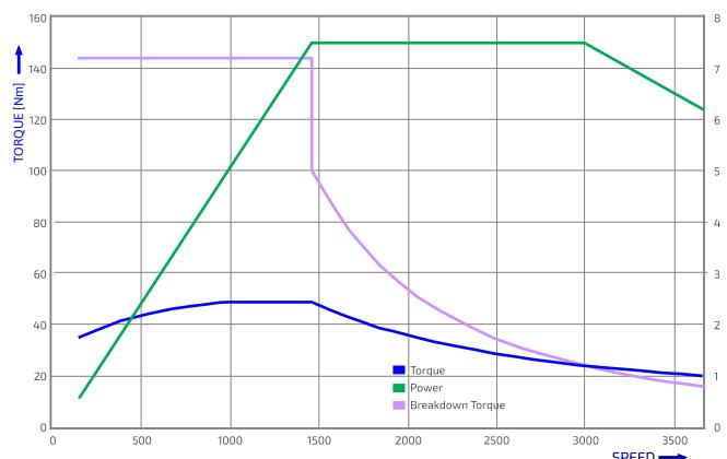
Where the 'Breakdown Torque' curve (violet) intersects the 'Torque' curve (blue) the range of "Constant Power" ends and after that the Breakdown Torque, which is decreased by 30% (to reserve for the Acceleration Torque), is the limiting Torque Value the motor can achieve.
