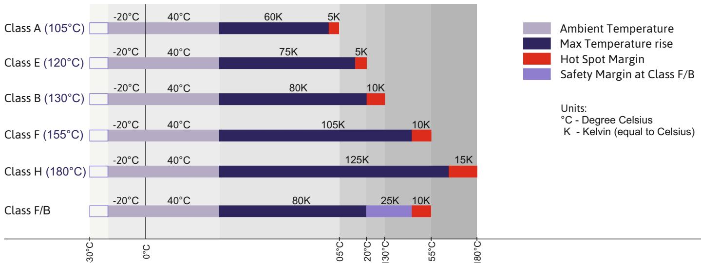
The maximum permissible temperature of the winding is determined based on the thermal class temperature limits. The temperature of the winding increases as a result of the copper and iron losses in the electric motor during operation. The winding temperature rise is determined through measuring the winding resistance, which increases with increasing temperature. To allow for any Hot Spots in winding lower temperature limits are specified for the insulation materials.
